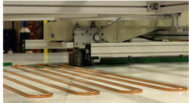
Picture 2: Atrium Plana high precision laser welding.
